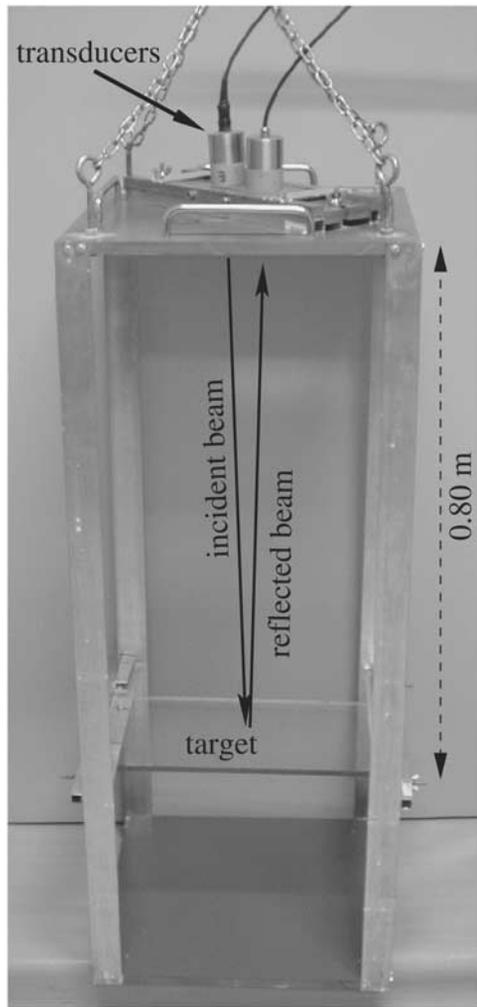
**Figure 10.** Experimental setup used to perform multiscale ultrasonic probings. The whole apparatus is immersed in a large water tank. Four pairs of transducers are used to span a frequency range from 150 kHz to 1.2 MHz. They are tilted in order to align their beams on a common incident spot. The targets are polyacrylate plates with thicknesses of 1, 2, 4, and 8 mm.
