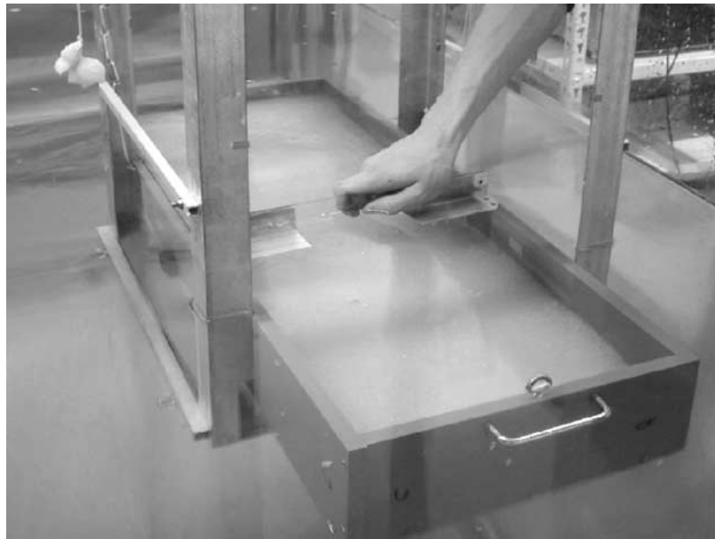
Figure 12. The surface of the granular medium constituted by glass beads is manually smoothed by translating a Plexiglas slab held vertically across the box. Two passes with the slab are sufficient to suppress surface irregularities larger than one bead diameter while avoiding any regular arrangement in the shallowest layers of beads.
