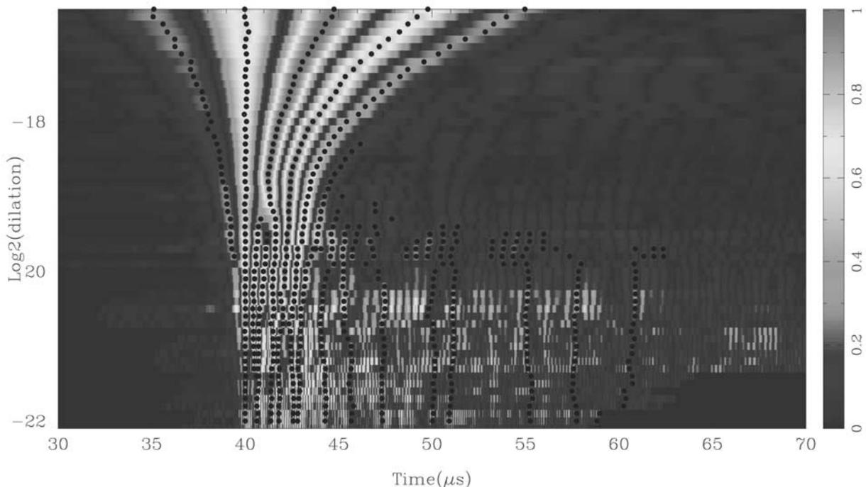
**Figure 13.** Modulus of the experimental wavelet response rescaled for glass beads with  $d = 1.1$  mm (see text for details). The black dots represent the lines of maxima associated with the ridge functions shown as symbols in Figure 14. The individual signals forming this noncausal wavelet response have been arbitrarily shifted in time in order to align their second relative maxima (dotted line of maxima labeled 1).
