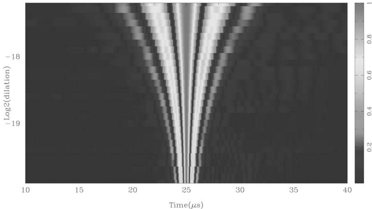
**Figure 9.** Representation of the modulus of a wavelet response obtained by propagating the source signals through water. The dilation  $a = f_c^{-1}$ , where  $f_c$  is the main frequency of the wavelets which are dilated versions of the fourth derivative of a Gaussian.
