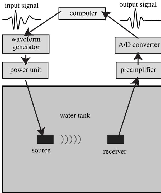
**Figure 7.** Schematic view of the setup used to construct the experimental wavelet response. A nonlinear inverse method (F. Conil, personal communication, 2002) is used to find the numerical input signal (top left) to send to the arbitrary waveform generator in order to obtain an output signal (top right) equal to a pure wavelet as the one shown in Figure 8.
