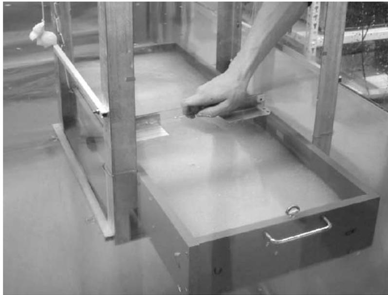
**Figure 12.** The surface of the granular medium constituted by glass beads is manually smoothed by translating a Plexiglas slab held vertically across the box. Two passes with the slab are sufficient to suppress surface irregularities larger than one bead diameter while avoiding any regular arrangement in the shallowest layers of beads.
