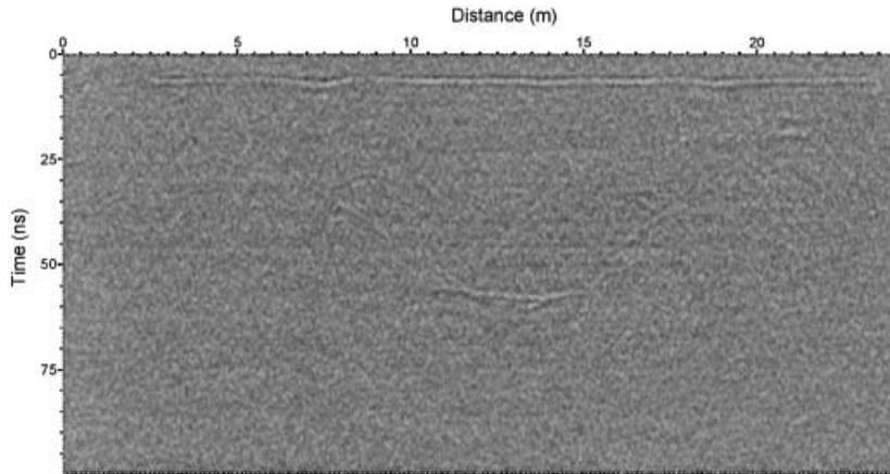
Figure 8 Random noise added to the GPR time-section acquired on the test site with two 500 MHz antennae and an offset of 0.75 m. The statistical distribution of the noise is Gaussian and was filtered between 20 MHz and 750 MHz.
