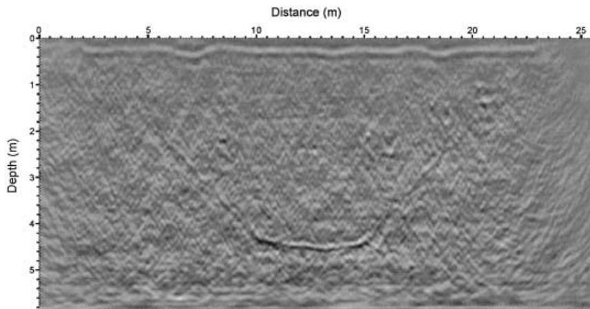
Figure 9 Migrated image of the noisy common-offset measurement shown in Fig. 8 with a migration velocity of 0.159 m/ns.
