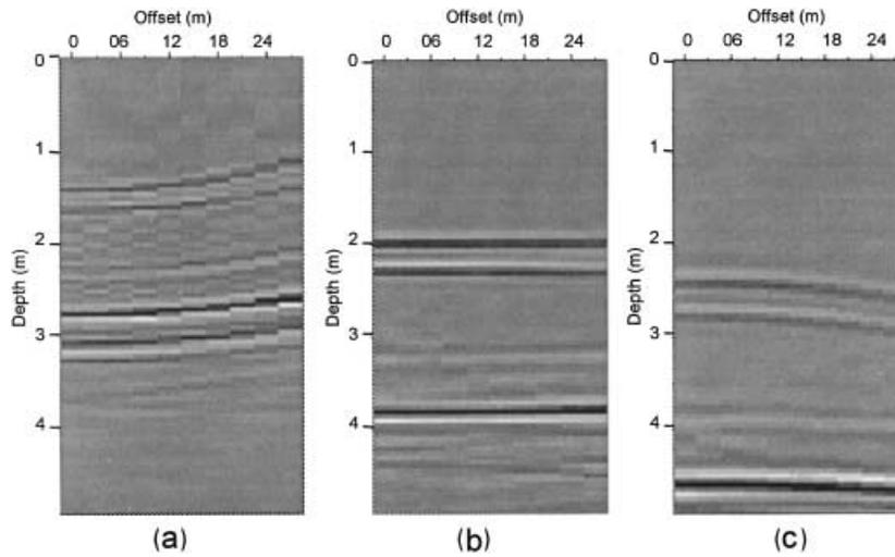
Figure 3 Panels showing common-offset migrated data obtained from numerical data similar to Fig. 2 data: (a) for a migration velocity of 0.11 m/ns; (b) for a migration velocity of 0.15 m/ns; (c) for a migration velocity of 0.18 m/ns.
