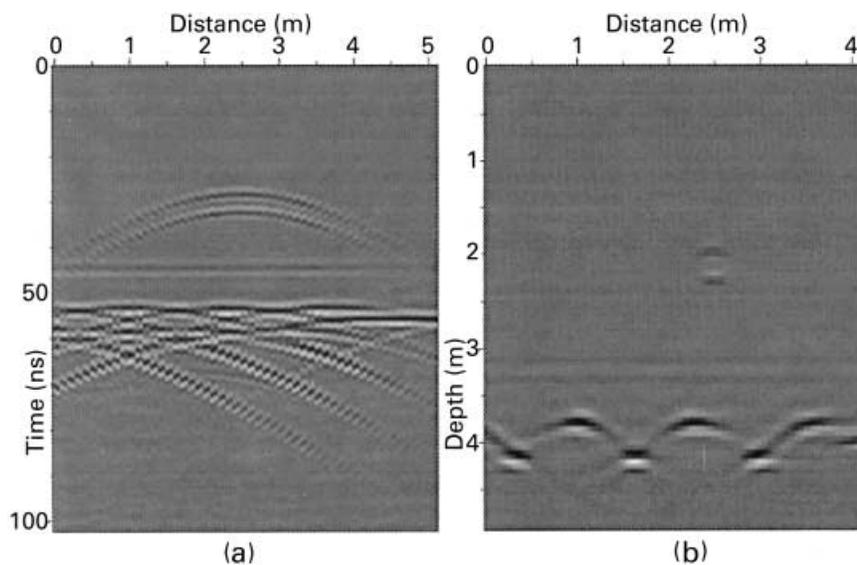
Figure 2 Prestack migration of a synthetic time-section. (a) Common-offset synthetic time-section. (b) Stacked migrated image from the different synthetic common-offset data (the offset ranges between 0 and 2.7 m).
