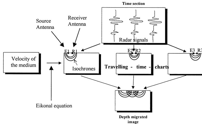
Figure 1 Diagram of the migration principle for a common-offset time-section acquired in a medium with constant velocity.
