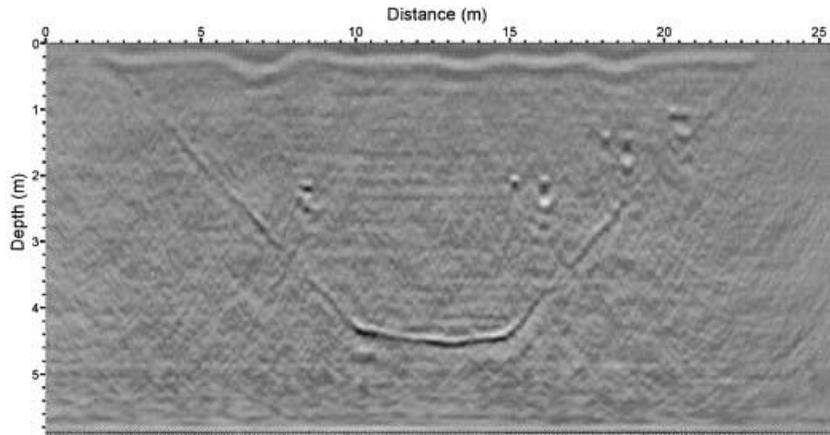
**Figure 10** Stack of migrated noisy common-offset measurements for several offsets (0.75 m, 0.85 m, 0.95 m, 1.15 m, 1.25 m, 1.35 m, 1.55 m) and a migration velocity of 0.159 m/ns.
