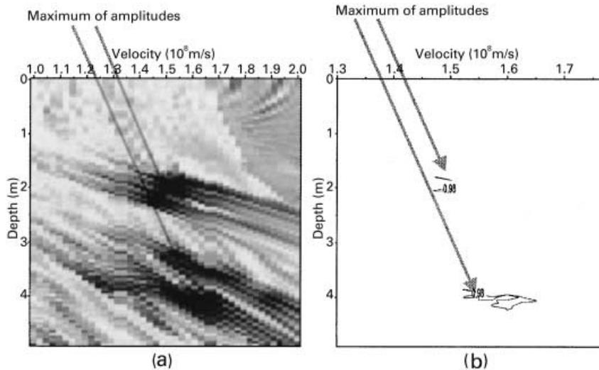
Figure 4 Semblance panel obtained from the several common-offset migrated data obtained using numerical data similar to Fig. 2 data: (a) contrasts image of semblance; (b) contours of semblance equal to 0.98.
