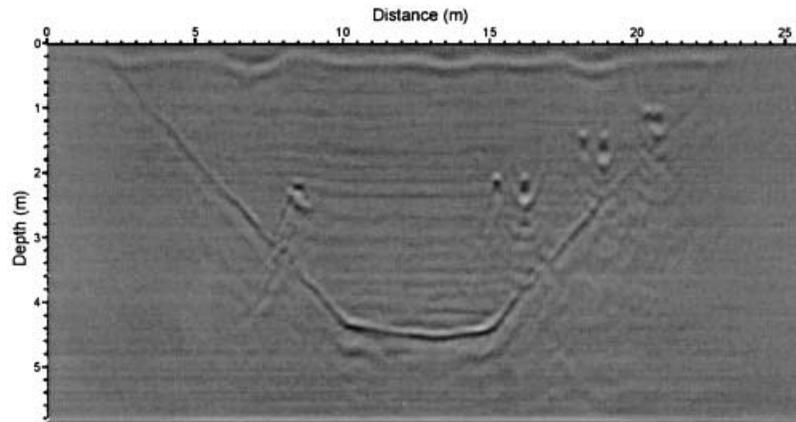
Figure 7 Stacked migrated test site measurements acquired with several offsets (0.75 m, 0.85 m, 0.95 m, 1.15 m, 1.25 m, 1.35 m, 1.55 m) and a migration velocity of 0.159 m/ns.
