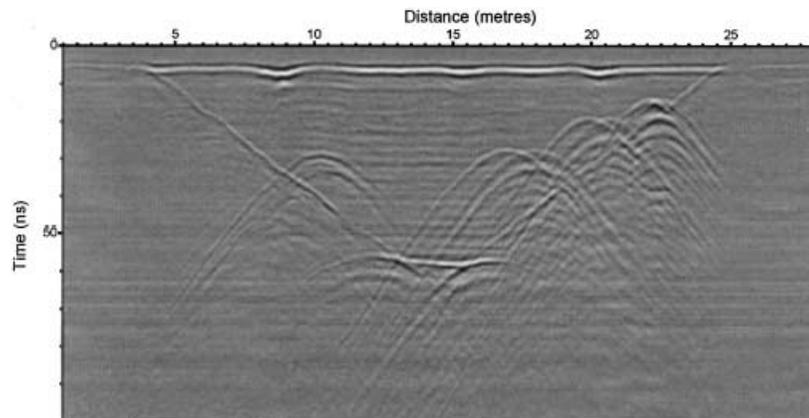
Figure 6 GPR measurements on the test site using two 500 MHz antennae and an offset of 0.75 m.
